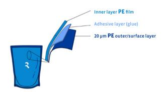
A **typical application**: a mono-material stand-up pouch consisting of All-PE films. A stand-up pouch is a widely used packaging solution. It usually consists of a PE layer on the inside, which is sealed at low temperatures. Typically, it is laminated against reverse printed PET on the outer layer. By replacing the PET with a stretched PE film, the packaging becomes fully recyclable.
