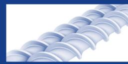
This is made possible by the twin-screw technology, which homogenizes the melt better and thus ensures a stable process. In addition you can degas the system very easily and effectively, removing unwanted components in the recyclate.
