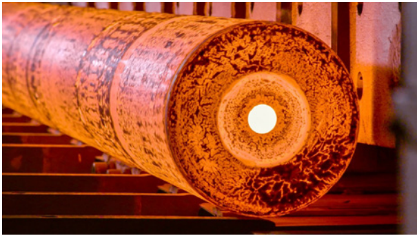
Armored barrels: 14-400 mm inner diameter up to 9 m length
